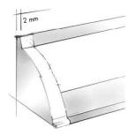
2. When attaching the lower splashback upstand, ensure that the worktop surface is predrilled in the screw fastening area. The holes must be at least 1 mm larger than the screw diameter to prevent stresses building up in the material. We also recommend protecting the inside of the screw hole with sealant before screwing.
