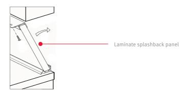
7. Close the profile ends with the supplied end caps and close the shadow gap between the rear edge of the laminate splashback panel and the wall with the side cover profile.
